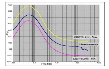
Isolation curve Terminal EUT RF connector terminated
