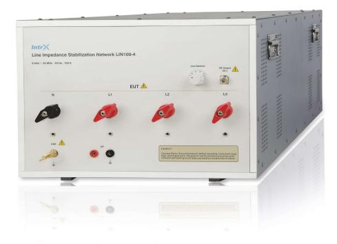
LISN (Artifical Mains Network) is a low-pass filter typically placed between an AC or DC power source and the EUT (Equipment Under Test) to create a known impedance as per complying standard for the measurement of conducted emission. It also isolates the unwanted RF signals from the power source with pre-filter included. It provides a Radio frequency (RF) noise measurement port.
