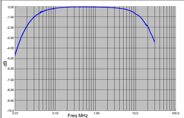
Impedance curve Terminal EUT RF
