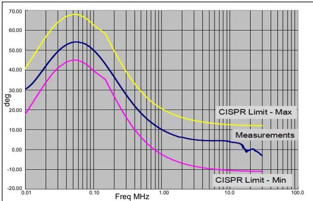
Isolation curve Terminal EUT RF
